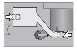
Release the cover to the milk pipework by pressing the tabs in on the left and right hand sides.
